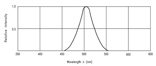
Fig.1 Relative Intensity vs. Wavelength
